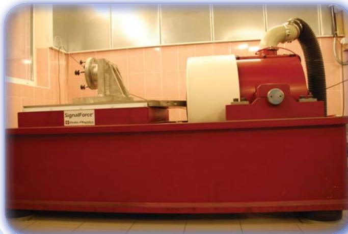
Вибростенд GW-V1322, Gearing & Watson Electronics,
